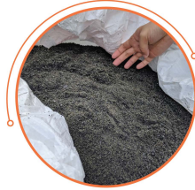
MSW Slag collected at the Tuas South Waste-to-Energy Research Plant.
