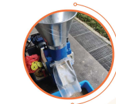
Pelletizing of fish feeds
