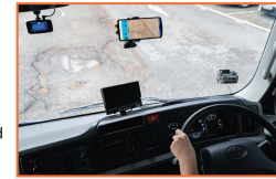
Phone is mounted on vehicle dashboard and photographs are captured while driving. (Photo credits: JTC)
