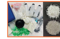
Mixed plastic feedstock processed into grinded forms for concrete footpath & asphalt road pavement
