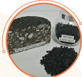
Cross section of asphalt with recycled plastic
