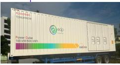
1 MWh Vanadium Flow Battery Storage of solar energy for use at night and for grid-forming.
