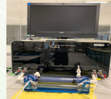
Fouling Evaluation System
