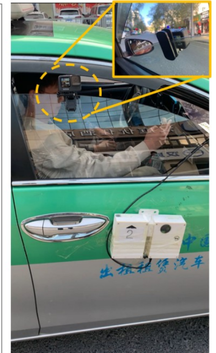
Task division for mobile sensing: simultaneous data collection and equipment installation on three taxis
